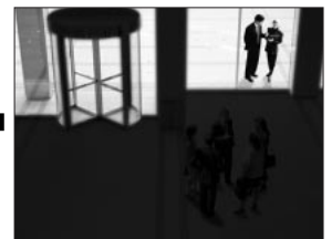
To view outside the iris must be closed but the image of the inside is too dark to see.
